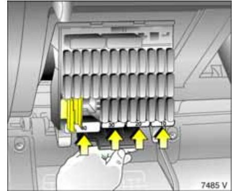
Only use fuses with the correct rating. This is shown on all fuses and is also indicated by the fuse colour.
