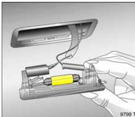
2. Press bulb slightly towards spring clip and remove.
