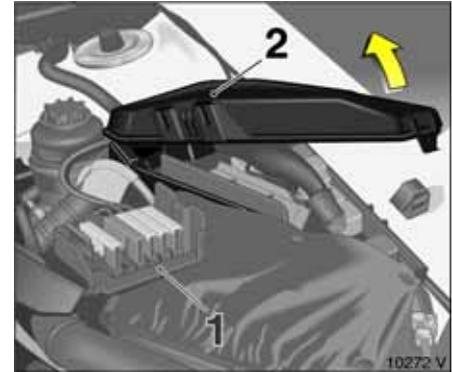
The fuses for the preheating system and fuel filter heating (diesel engine), as well as other relays and fuses depending on vehicle equipment, are located in the fuse and relay box 2.
