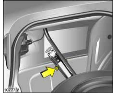
In vehicles with towing equipment \* the jack is stowed behind the spare wheel. It is secured with a wing screw. Spare wheel – see next page.
