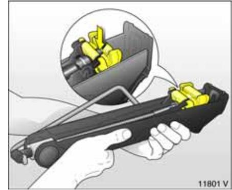
4. Before attaching the jack, set it to the required height by hand. Fit the jack arm – at the front or rear – in such a way that the jack claw (arrow in figure) goes around the vertical ridge and engages into the recess in the ridge.
