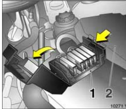
**Fuses in the engine compartment**
