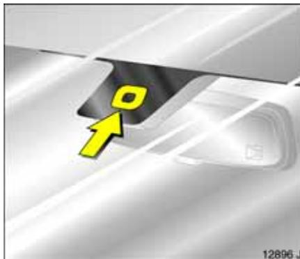
So as to ensure proper operation of the rain sensor \*, the sensor field must be free from dust and dirt and the windscreen wash system must be operated at regular intervals. Vehicles with rain sensor \* can be identified by the sensor field near the top of the windscreen.
