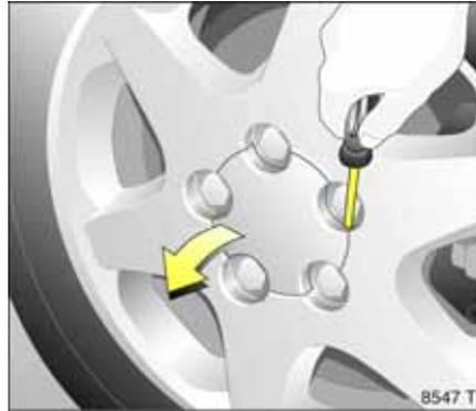
Alloy wheels ✱: Prise off the hub cap using a screwdriver, positioning the screwdriver at the recess at the side of the hub cap.
