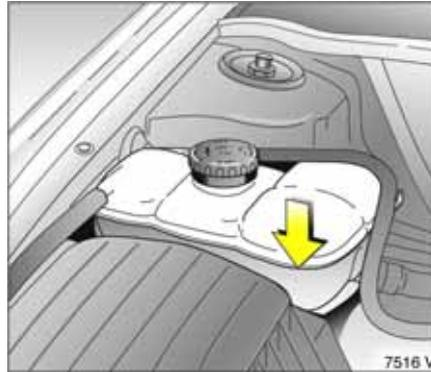
The coolant level in the expansion tank should be slightly above the **KALT/COLD** mark when the system is cold. It rises at engine operating temperature and drops again when the engine cools down. If the level falls below the mark, the coolant should be topped up to a little over the mark.
