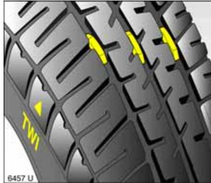
The legally permissible minimum tread depth (1.6 mm) has been reached when the tread has worn down as far as one of the wear indicators (TWI<sup>1)</sup>). A number of wear indicators are spaced at equal intervals around the tyre within the tread. Their position is indicated by markings on the tyre sidewall.
