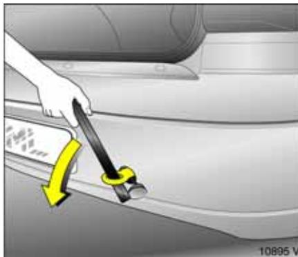
Screw in the towing eye anti-clockwise as far as it will go and use the wheel bolt key to tighten it until it is fully horizontal.
