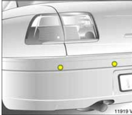
The system registers the distance by means of four sensors on the rear bumper. To ensure that the sensors function correctly and that the information provided is correct, they must be undamaged and free of dirt, snow and ice.
