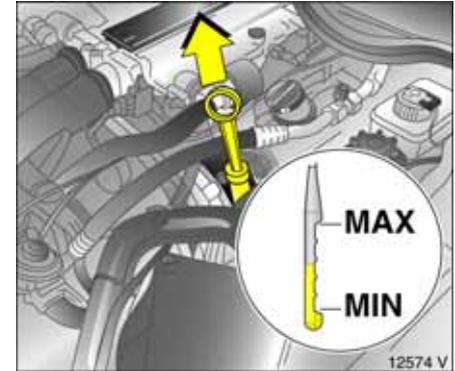
To check the level, remove the oil gauge (dipstick), wipe it clean and reinsert it as far as it will go. Top up if the oil level has dropped to just above the "add oil" mark **MIN**.
