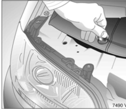
To change front headlamp bulbs, remove relevant cover: turn rotating lock through 90° using a coin and remove cover.
