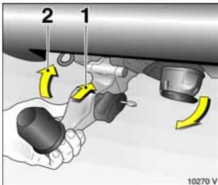
Insert front end of coupling ball bar into coupling housing (1) and swivel rear end upwards (2) until coupling ball bar engages audibly in coupling housing.
