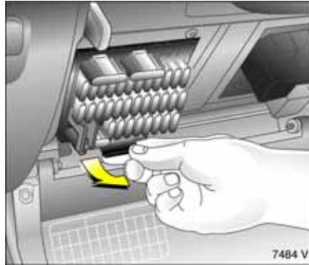
To replace a fuse, grip handle to disengage fuse box from underneath and swivel forwards.
