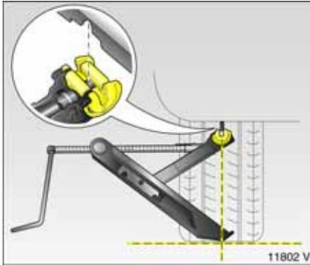
When turning the crank, ensure that the edge of the jack base on the ground is vertically in line with the contact point.
