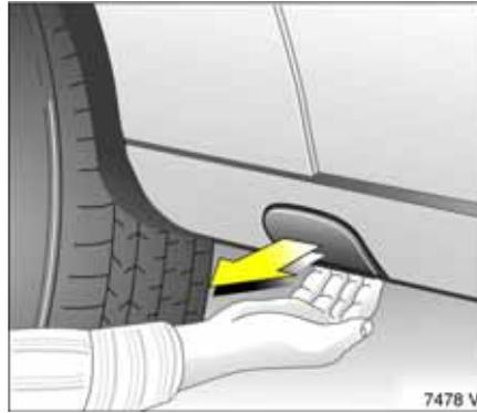
3. Depressions concealed by flaps at the front and rear on the vehicle underbody indicate the points where the jack is to be attached. Fold the flaps outwards to access the jacking points.
