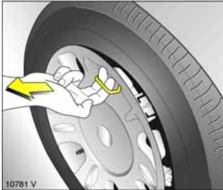
1. Prise off the wheel cover using the hook included with the vehicle tools. Vehicle tools – see page 179.
