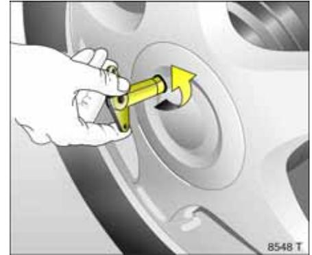
Alloy wheels with anti-theft lock ✱: Release hub cap using key included in vehicle tools and remove it.
