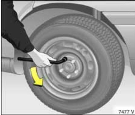
2. Loosen wheel bolts using wheel bolt wrench.
