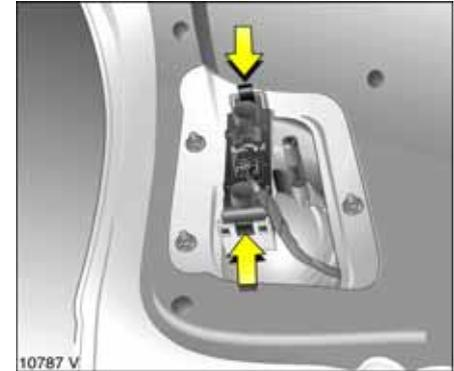
Press retaining lugs at top and bottom of bulb mounting inwards and remove bulb mounting.
