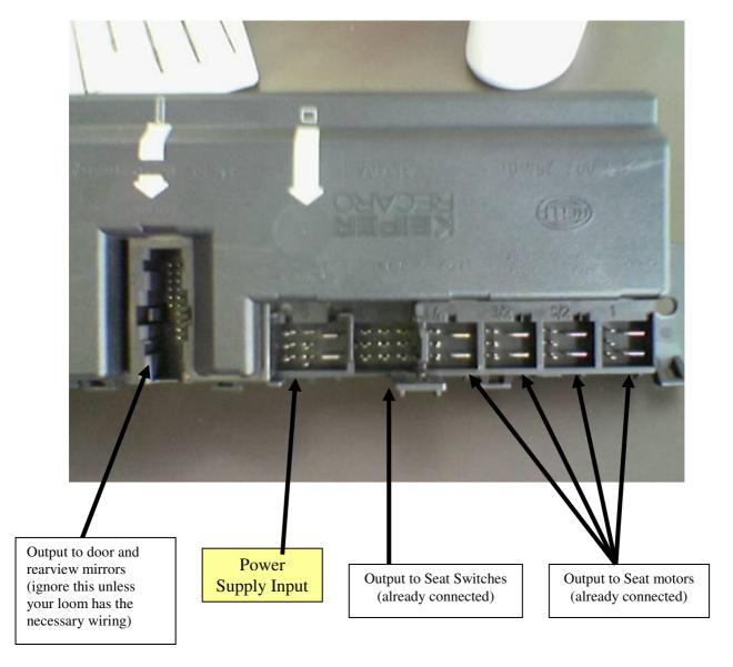
try and get a matching plug for the power feed connector if possible (marked as number 6 on the box) - connect feed and earth wires as follows...
