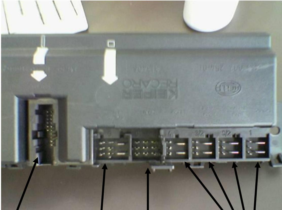
Output to door and rearview mirrors (ignore this unless your loom has the necessary wiring)
